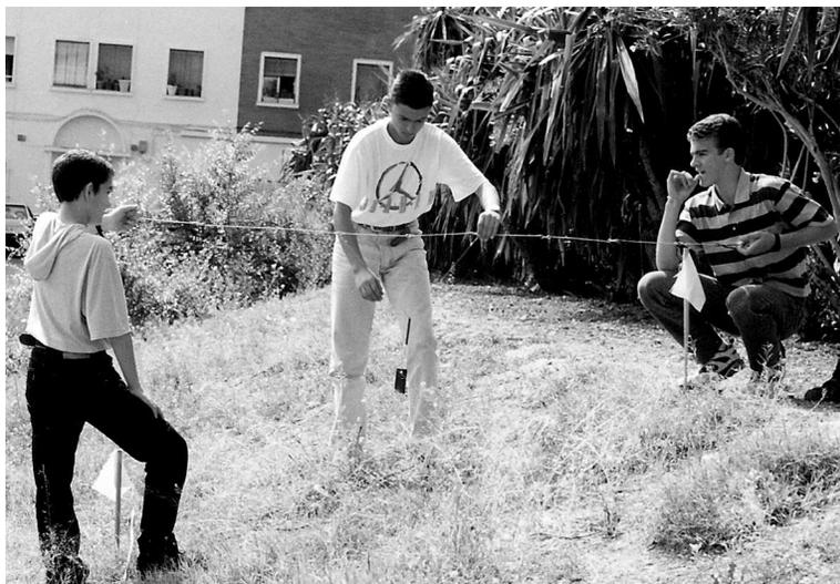
**Figure 11.5.** Measuring a tract of land using a surveyor's chain.
